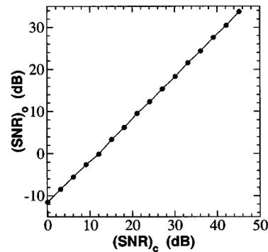
Fig. 7. Synchronization performance of the chaotic optoelectronic feedback system indicated by  $(SNR)_e$  versus  $(SNR)_o$ .
