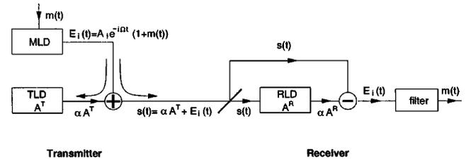
Fig. 1. Schematic setup of message encoding and decoding with additive chaos modulation in an optical injection system.
