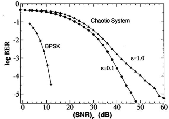
Fig. 4. BER versus  $(\text{SNR})_c$  of the chaotic optical injection system. The BER of a BPSK system is also shown for comparison.
