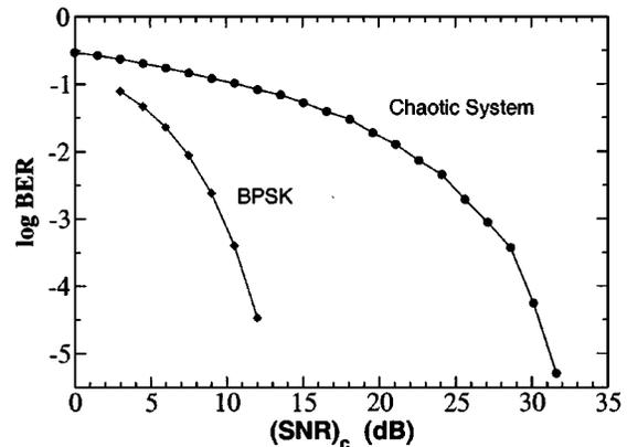
Fig. 8. BER versus  $(SNR)_e$  of the chaotic optoelectronic feedback system. The BER of a BPSK system is also shown for comparison.
