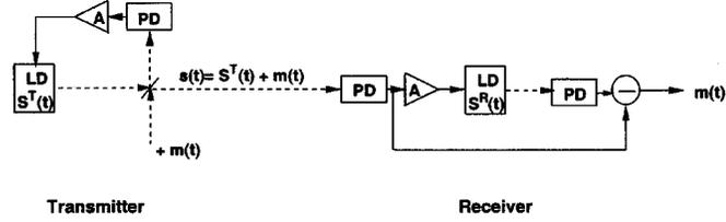
Fig. 5. Schematic setup of message encoding and decoding with additive chaos modulation in a delayed optoelectronic feedback system. Dashed lines show the optical paths.
