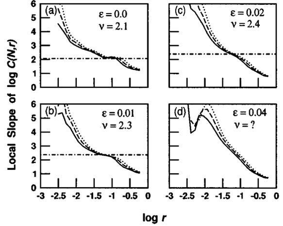
Fig. 6. Calculated correlation dimension plots with different message amplitudes in the optoelectronic feedback system.
