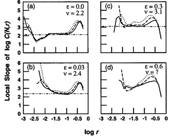
Fig. 2. Calculated correlation dimension plots with different message amplitudes in the optical injection system.
