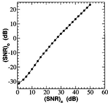
Fig. 3. Synchronization performance of the chaotic optical injection system indicated by  $(\text{SNR})_c$  versus  $(\text{SNR})_o$ .
